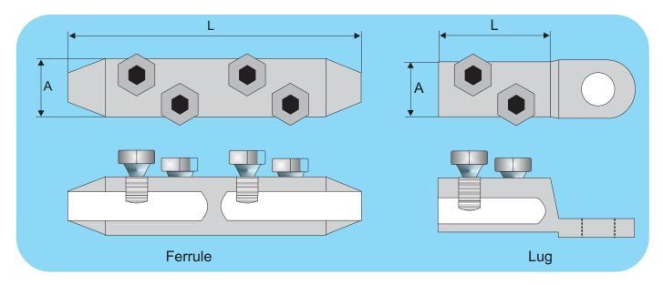
JOINTMASTER now offers a comprehensive range of mechanical torque shear connectors for use on both round, compacted and sectoral copper or aluminium conductors. These connectors utilise an offset bolt configuration that results in maintaining a much shorter length than traditional mechanical connectors.
